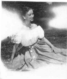
NEGATIVE ROLL LIGHT-STRUCK IN LOADING Note white streaks across picture. Do not break transparent tape seal!
